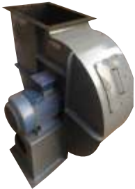
FIG C. Blower Impeller directly fitted with the shaft of Pedestal mounted motor. Generally used in Exhaust of Air, Spray booth (dry/wet) & Cyclone Exhaust, Dust Collector Bag-filters etc.
